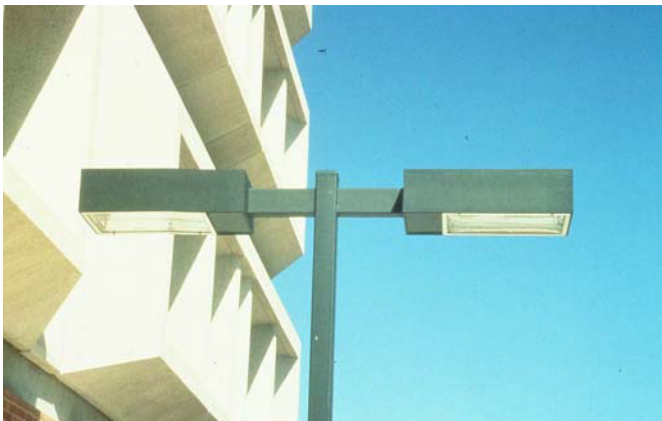
An example of a full cutoff low pressure sodium fixture.
